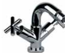
25CR0532 01 Miscelatore bidet. One hole bidet mixer. 3/8" 25 CR 0532 01 = flex 3/8"F 1/2" 25 CR 0532 02 = flex 1/2"F
